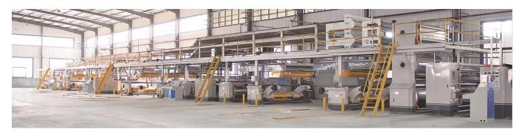
Corrugated Cardboard Production Line is the professional equipment for producing corrugated cardboard. The 3ply, 5ply, 7ply and multi-function corrugated cardboard production line mainly consist of the following equipment: Mill Roll Stand, surface paper (core-paper) pre-heater, single facer, Conveying Bridge, Glue Application Machine, Double Facer, Slitter Scorer, Cut-off, Conveyer and Stacker, Heating System, Air compression system and Glue Making System, etc.
