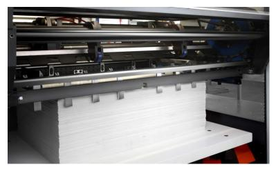
Delivery section add tester into security system. It is equipped with inset counter. Using subsection could adjust brush and sheet air-blowing device, so the finished product of delivery section could product stably. Gripper drive train expanded buffer device. NON-STOP PAPER DELIVERY BRING HIGH RETURN!
