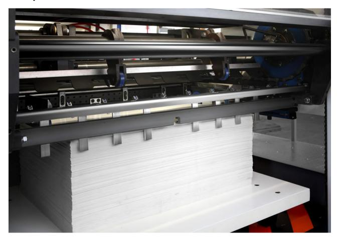
Delivery section add tester into security system. It is equipped with inset counter. Using subsection could adjust brush and sheet air-blowing device, so the finished product of delivery section could product stably. Gripper drive train expanded buffer device.
