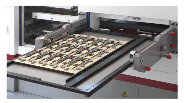
The driving gear ensures high speed of die cutting together. The pneumatic locking mechanism and air clutch are fast and stable. The die cutting frame can prevent the die cutting plate from drooping or separating effectively.
