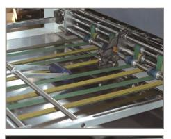
\* Unique Pressing Transferring Unit, the board are transferred under pressure from the roller. And it avoid the crash between the roller and board.
