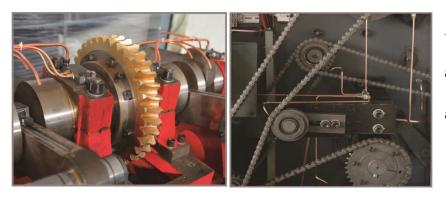
All the key moving parts, chains and touch points are lubricated automatically by central oil pump.
