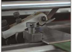
\*Side lay has two functions, pushing and pulling which can be adjusted according to the board.
