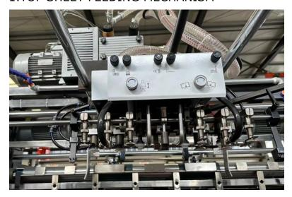
High precision high speed automatic feeder, , feeding smoothly.
