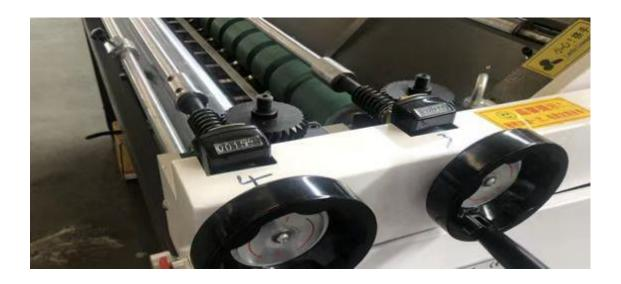
Single pressure regulation, to ensure that the two side pressure be same With the display of dial gauge, it is easy to adjust when change the paper
