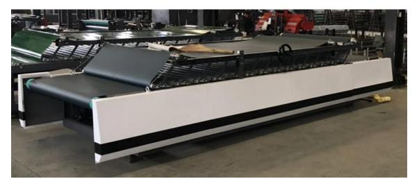
Floating design of press, no need to adjust the pressure Heightening design, smooth working for thick corrugated paperboard
