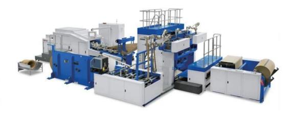
It is a one-time automatic production of paper bags with round rope handles by using printed roll paper as raw material, combined with handle paper sheets and paper ropes.
