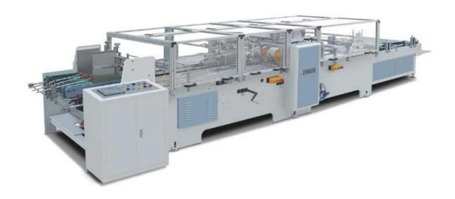
Handbag bottom-gluing machine features a continuous function of automatic delivery of manually-folded bag bottom (paperboard can inserted or not), automatic water-soluble glue, automatic pasting, automatic folding, pressing and finished bag bottom output. This machine adopts touch-screen operation, photoelectric switch. The user can adjust the glue thickness and length according to requirements. With high precision and speed, this machine can produce various specifications of bags.
