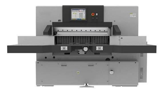
Japan Hydraulic components, Japan, Korea electrical components, Taiwan ball lead screw, Linear double guide rails, PLC control system are adopted to monitor all mechanical implementation. Its key parts adopt imported bearing of low maintenance.
