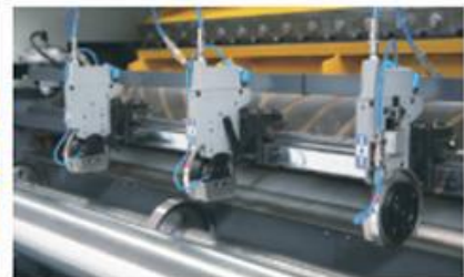
Three sets of slitting knife are used for trimming and middle slitting.
