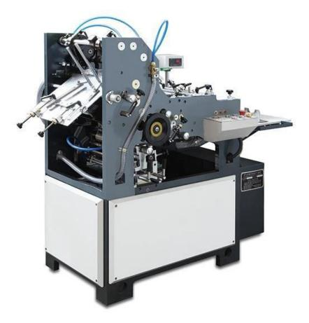
HP-250 Full automatic packet envelope making machine is suitable for producing small pocket envelope (open-end envelope), red pocket, chopstick bag, drug bag and so on.
