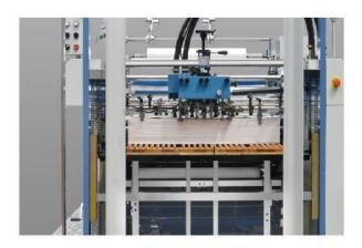
This machine is equipped with a paper pre-stacker, Servo controlled feeder and a photoelectric sensor to ensure that paper is continuously fed into the machine.
