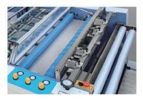
Pneumatic separation system to separate the paper stably and quickly.
