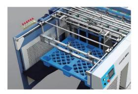
Automatic stacker receives the sheets quickly in order without stop the machine as well as counter the sheets
