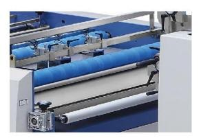
The machine is equipped with an anti-curl device, which ensures that paper remains flat and smooth during the lamination process.
