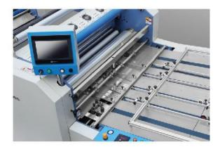
A user-friendly interface system with a color touch-screen simplifies the operation process. The operator can easily and automatically control paper sizes, overlapping and machine speeds.
