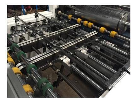
2) The paper moving system adopt pushing chain and air sucking belt. They have positioning function, insure the paper comes same place in same time.
