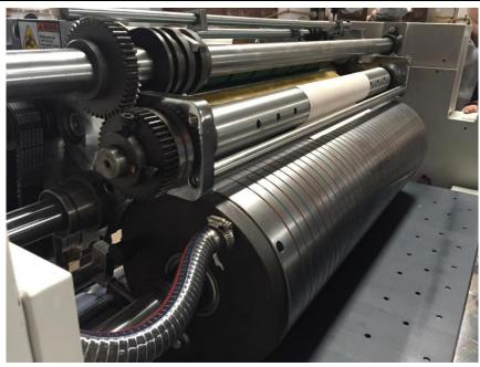
4) The film cutting part adopt roll-knife. It is controlled by servo motor so that we can adjust the film length without stop in the PLC. It also can adjust the place of film on the paper without stop. It has special knife to cut film for tissue box.
