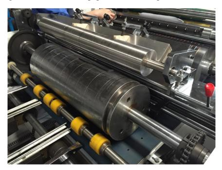
3) Glue part adopt flexo printing technology. We can adjust the place of glue on the paper without any stop. When missing paper, glue part will up in case of the glue leaves on the air sucking belt.
