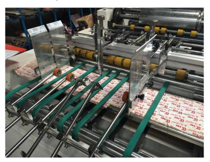
1) The paper feeder is controlled by servo motor, the belt is from Poland. No-stop feeding paper, no overlapping paper or missing paper.
