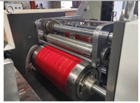
4) The film cutting part adopt roll-knife. It is controlled by servo motor so that we can adjust the film length without stop in the PLC. It also can adjust the place of film on the paper without stop. It has special knife to cut film for tissue box.
