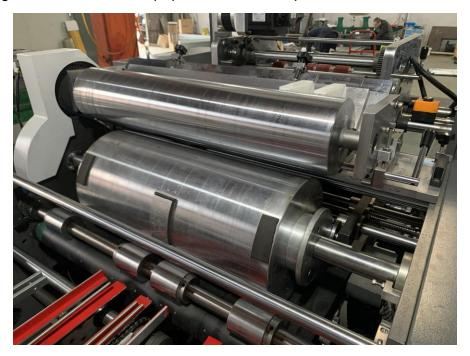
3) Glue part adopt flexo printing technology. We can adjust the place of glue on the paper without any stop. When missing paper, glue part will up in case of the glue leaves on the air sucking belt.
