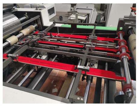
2) The paper moving system adopt pushing chain and air sucking belt. They have positioning function, insure the paper comes same place in same time.
