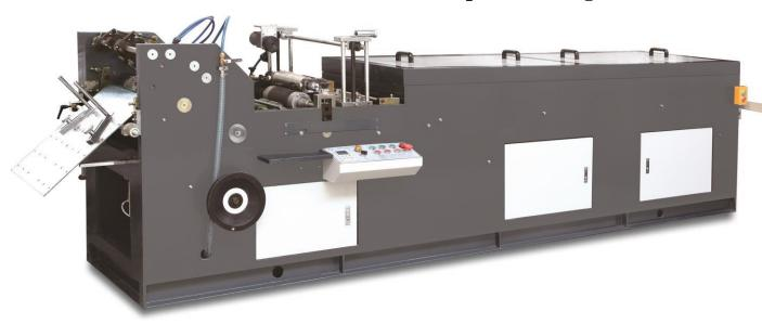
TJ-392 Full automatic self-seal envelope gumming machine is suitable for gumming remoist-enable adhesive on the seal flap of blank envelopes.
