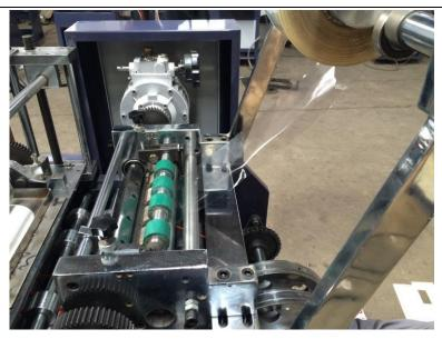
Adopting the automatic gear shifting to adjust the length of the film and high-speed accurate automatic film sticking unit
