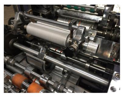
The gluing parts adopt the adjustable parts gluing structure, it is convenient for adjustable according to the paper requirement and the gluing position, save the gluing quantity, it is easy for pulling out the gluing parts, convenient for washing.
