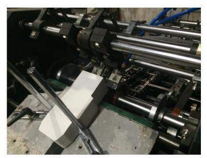
The air-suction bottom feeding system ensuring the automatic feeding of non-stop operation of the equipment
