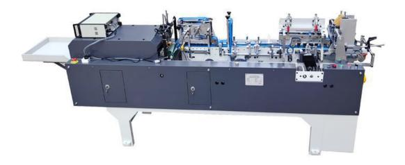
ZH-500 mini automatic folder gluer is the Company's latest economic and flexible type of small folder gluer, the aircraft are small but fully functional, with automatic feeder, automatic gluing, automatic folding, automatic counting, and other functions. It is the small and medium-sized printing factories required equipment.
