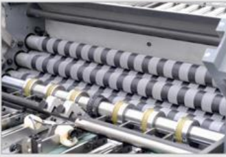
胶辊采用国际先进技术压注 Cast Rubber Roller Of International Advanced Technology
